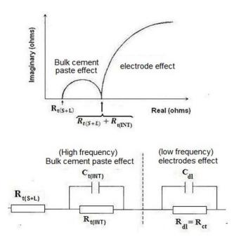
Figure 2: a) Schematic of EIS spectra of concrete, b) Equivalent electrical circuit for concrete [4].
