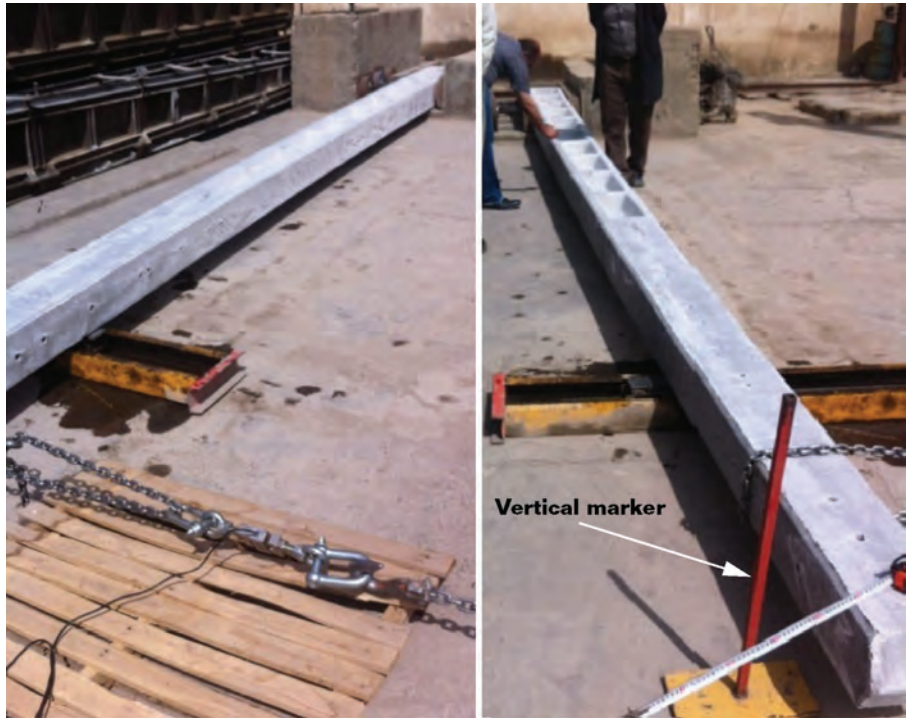
FIGURE 1 Position of the concrete pole and the steel marker during the bending test.
