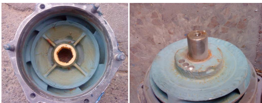
FIGURE 2 A polymer composite coating prevented cavitation and erosion in a pump with 18 months of operation.
