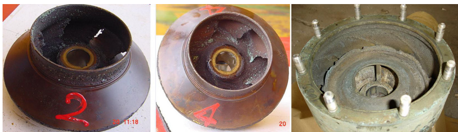
FIGURE 1 Cavitation damage to an impeller and casing of a pump after about one month of operation. The pump was used for seawater injection in Iranian oil wells in the Persian Gulf.
