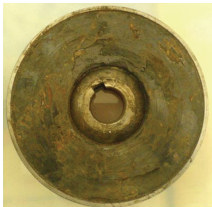
FIGURE 5 The rough and damaged surface of a thrust bearing carbon pad.
