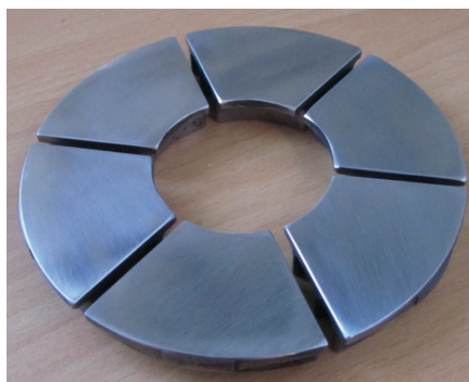
FIGURE 6 The finished surface of the SS pads after machining and polishing.
