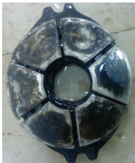
FIGURE 4 After the surface of SS segment becomes rough, carbon particles from the carbon pad fill in roughness voids and produce additional friction-related wear.
