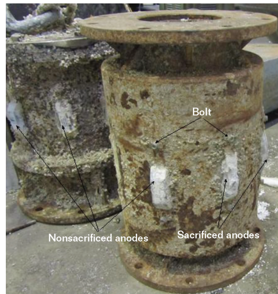
FIGURE 2 Sacrificed and nonsacrificed zinc anodes after six months of immersion in seawater.
